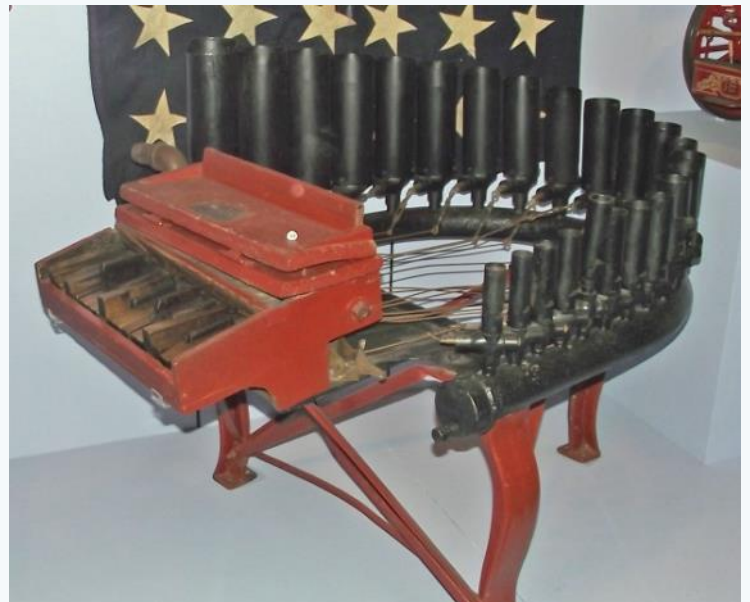
Steam calliope (c. 1901) built by George Kratz and used on the showboat French's New Sensation at The Mariners' Museum
