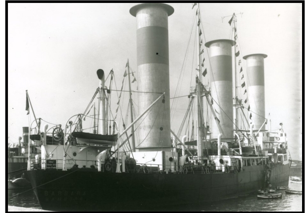
The Barbara, designed from the ground up with Flettner's rotorsail technology in mind
