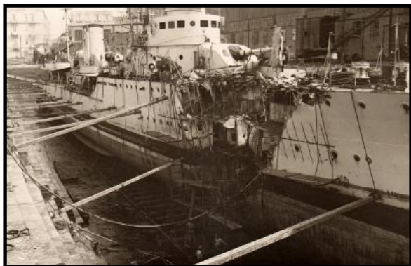
Antonio Usodimare in the dock after a collision with the steamer Pallada, September 1934
