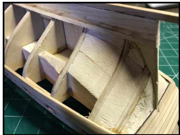
Detail of Blocking between bulkheads in Sean Maloon's Siren
