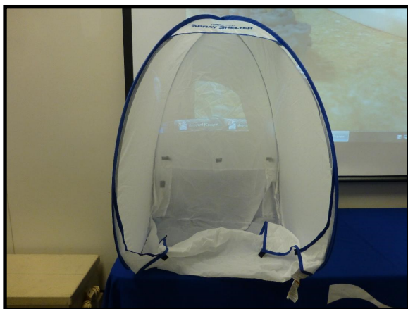
Yves Pochard's collapsible spray paint enclosure
