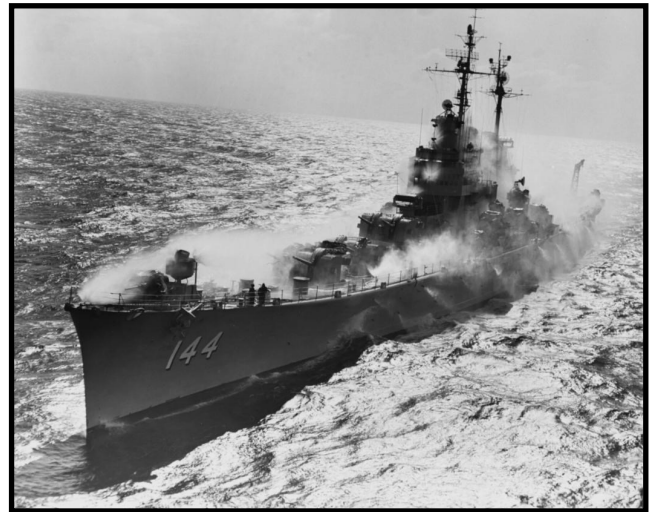
USS Worcester (CL-144) Testing her anti-nuclear radiation "washdown" system, 7 July 1954.
