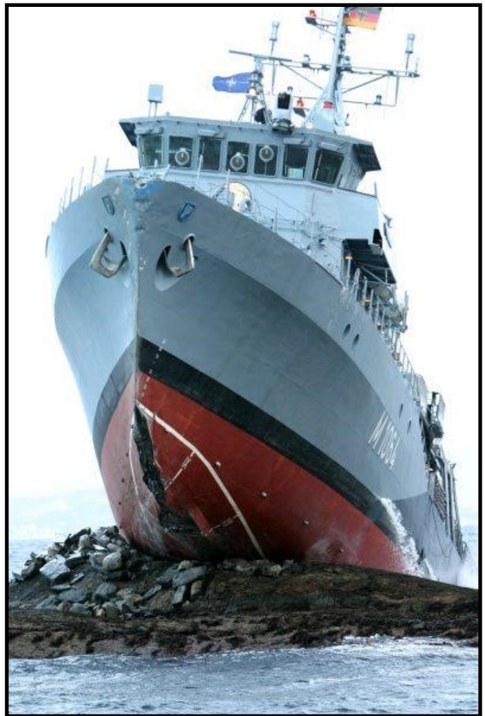
Showing bow damage on the Gromitz
