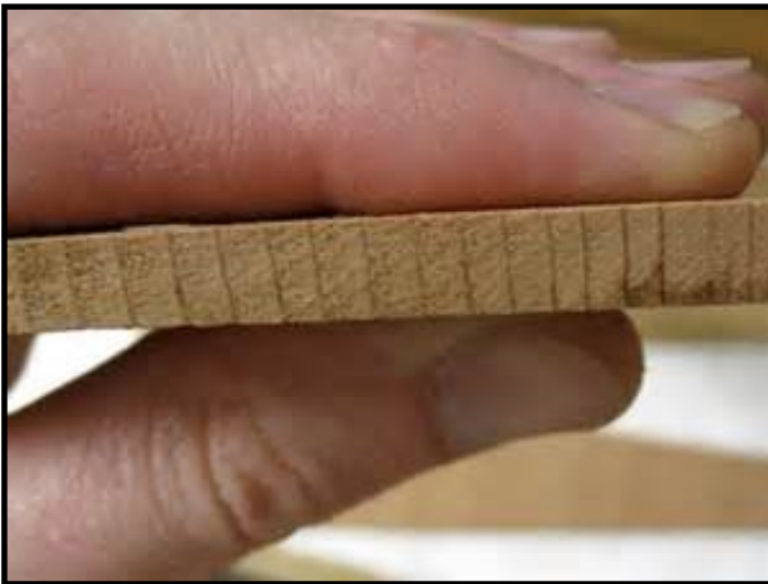
Grain direction of quarter sawn wood
