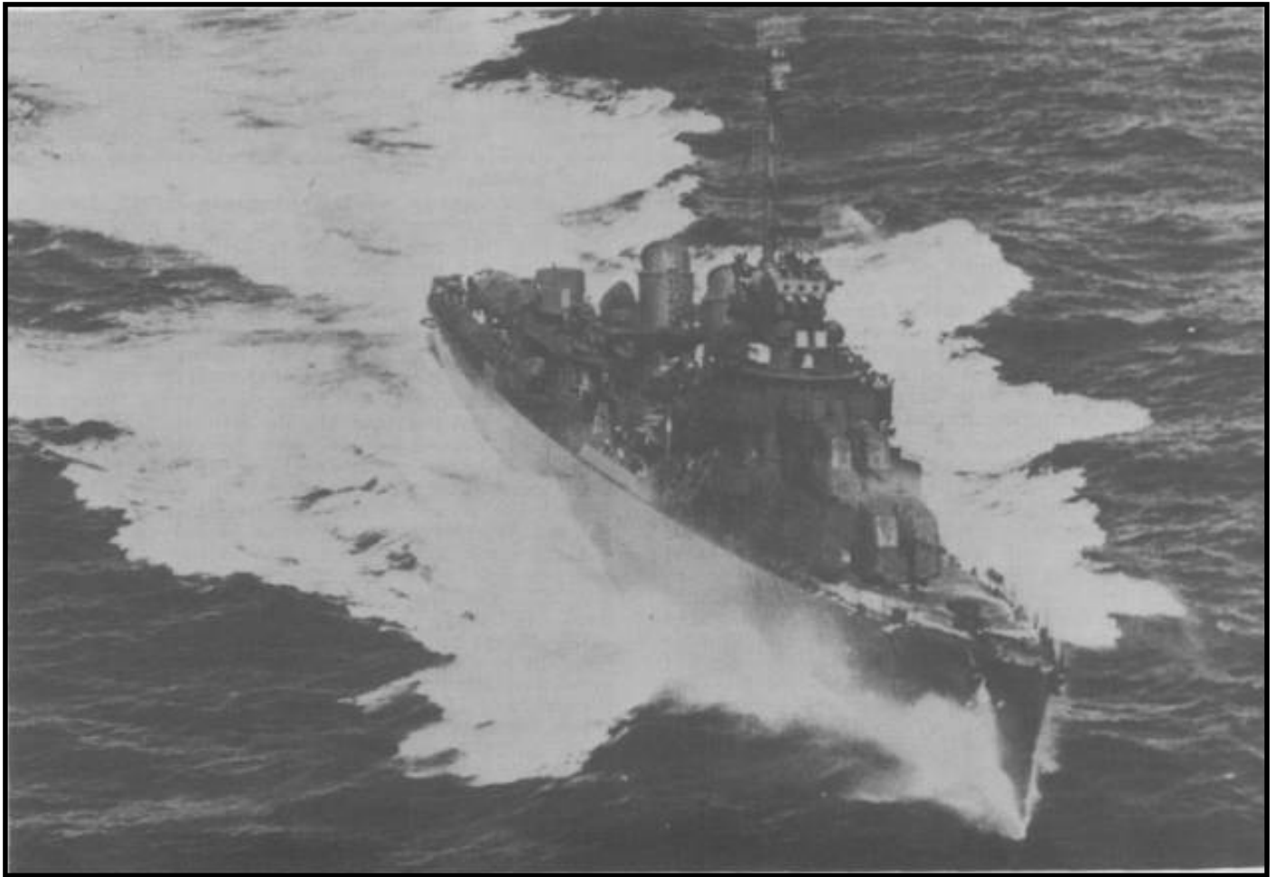
USS Stevens (DD-479), 1943. A catapult for launching an observation plane is mounted aft of the stacks in place of the fifth 5-inch gun mount normally installed in this class.
