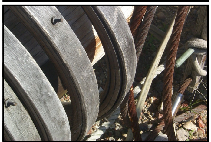
Detail of mast hoops on a Chesapeake Bay Skipjack
