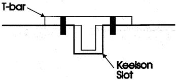
The T-bar slot can be made by cutting a longitudinal rabbet (in the top flat stock) using multiple passes on a small table saw. An alternate method is to cut the rabbet with a router bit mounted either in a router or a drill press. Run the drill press at its highest speed and mount a strip of timber on the drill press table to act as a guide, to assure a straight cut. Be sure that the T-bar ends up below deck level.
