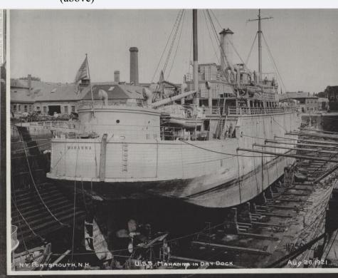
shows a freighter that is slightly different than the more familiar Ferris type 3-island steamer we are accustomed to seeing. The vessel measured 288 feet x 45 feet x 28 feet and was on par dimensionally and in cargo capacity with the Ferris type. The hard chine in the hull should have made for a more efficient cargo space.
