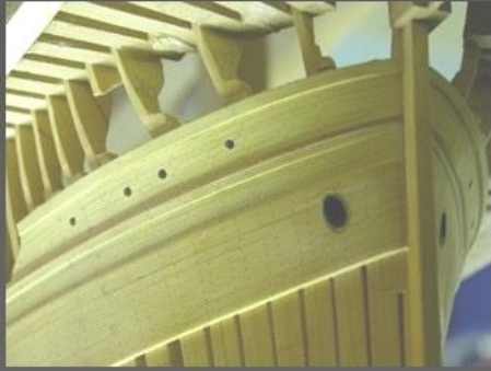
Finishing the Fo'castle Deck Beams & Hawse Pipes June 2007
