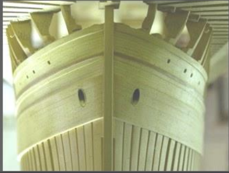
Finishing the Fo'castle Deck Beams & Hawse Pipes June 2007
