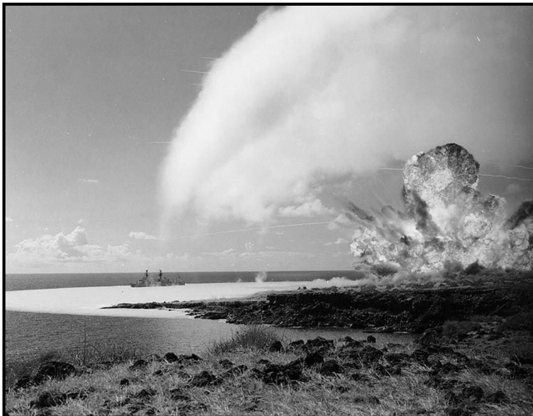
Detonation of the 500-ton TNT explosive charge for Shot "Bravo", first of a series of three test explosions on the southwestern tip of Kahoolawe Island, Hawaii, 6 February 1965. Weapons effects test ship *Atlanta* (IX-304) is moored in the left center. Note the shock wave spreading over the water just beyond the ship, and the shock condensation cloud lifting overhead.
